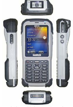
The design of the housing is elegant, clean and functional. There are hardly any visible screws and no small parts or details that look like they could break off. The entire device feels solid and capable of standing up to hard use. Note that the black bumpers serve as design elements as well as for protection. They seem glued on and it's not clear if they are meant to be replaceable should they get damaged.
