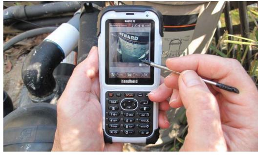
The sunlight-readable display measures 2.8 inches diagonally—a bit small perhaps considering that even tiny cameras now have 3-inch displays and larger and the trend in smartphones has been 3.5-inch and larger. It's a conventional resistive touchscreen that can be operated with a finger or the supplied stylus. The backlit 22-key phone-style keypad with smaller alphanumeric lettering includes a navigation diamond as well as ten(!) function keys and a dedicated scan key.
