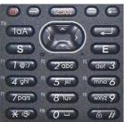
physical keypad, and it can be used for entering text as well. It's an expanded cellphone layout with some additional keys. The numeric keys that also access numbers, letters
