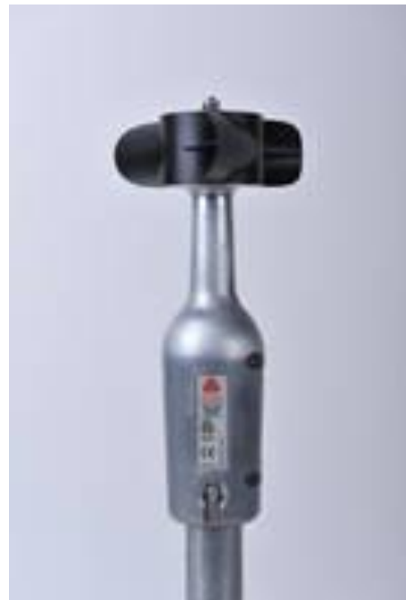
Slide sensor down over mast.
