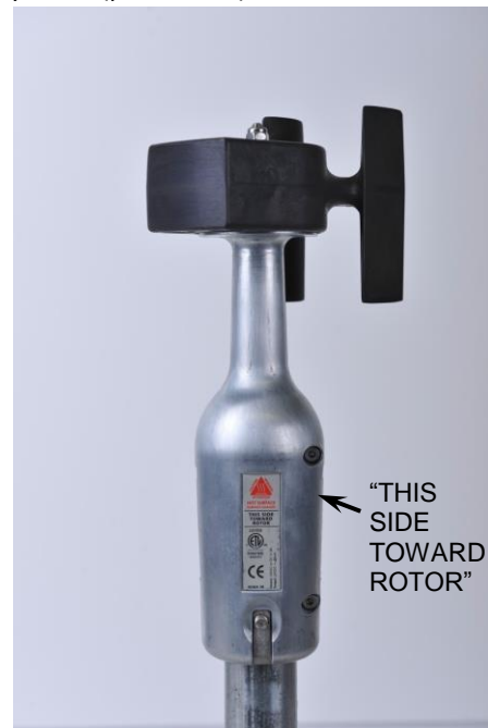
Slide sensor down over mast.
