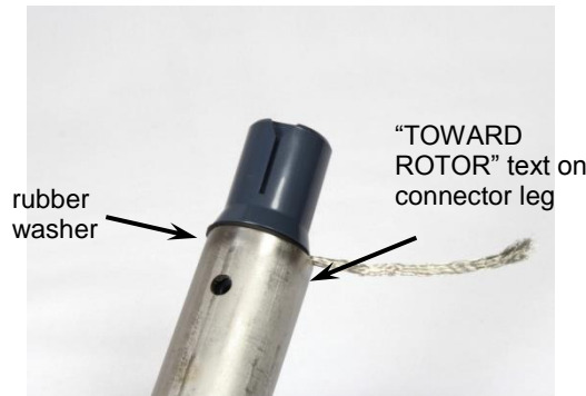
Install connector with "TOWARD ROTOR" text pointing to the rotor.
